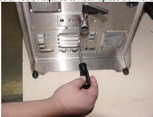
Figure 2: Removing Jack Screws
