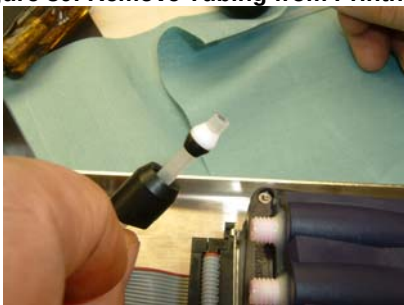
Figure 81: Do Not Remove Black and White Fittings
