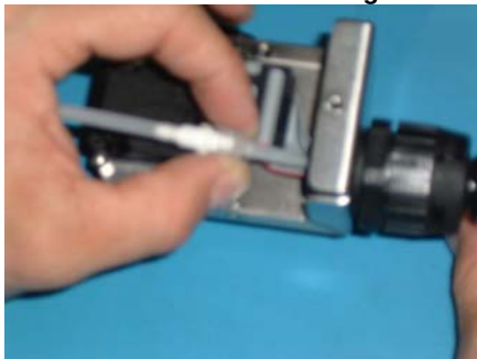
Figure 123: Disconnect Lure Fittings
