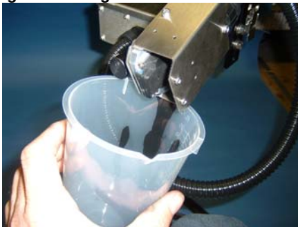
Figure 115: Priming into Container
