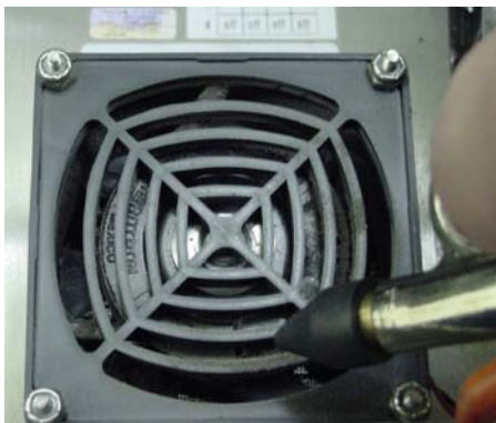
Figure 68: Blow Out Fan
